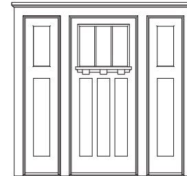
Main door with sidelights
